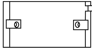
CB-973P(U) (205110P) Two oil holes 20° from split.
